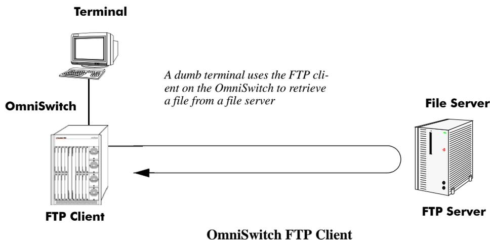
Use the switch **ftp** command to start its FTP client.
