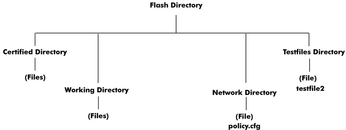
In this first example, the user's current directory is the flash directory. The following command syntax moves the **testfile2** file from the user created testfiles directory into the working directory as shown in the illustration above. The screen displays a warning that the file is being renamed (or in this case, redirected).
