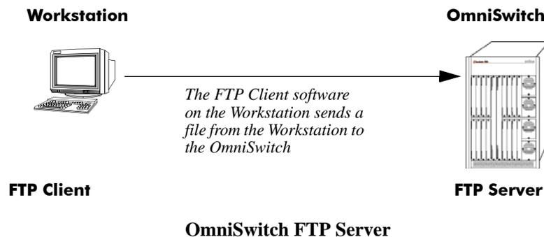
The following describes how to transfer files where the switch is acting as an FTP server.
